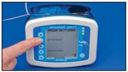
6) Power the pump on. Select "Keep Settings" to continue with previous setting or "Clear Settings" to start with programming new pump settings.
