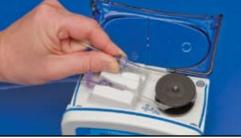
2) Grasp black ring retainer, gently wrap tubing around rotor, and insert retainer directly into right pocket. Do not overstretch tubing.
