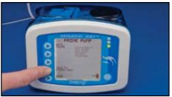
8) Press and hold the "Hold to Prime" button until only clean water flows through the tubing. Once the rotor starts this takes between 1 and 2 minutes.
