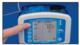
7) Press the "Prime Pump" button to enter the "Prime Pump" screen.
